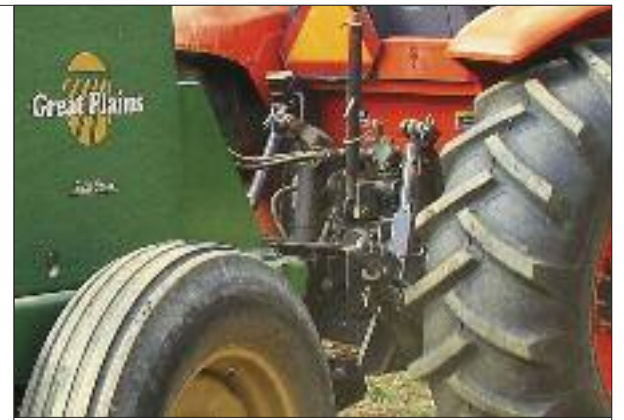
Drills are pulled by the tractor's drawbar.
