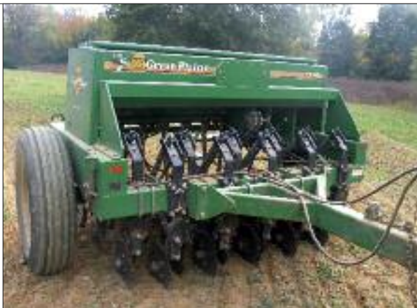
Unlike broadcast seeders, which throw seed out in an arc, drills place seed precisely in or on the seedbed.
