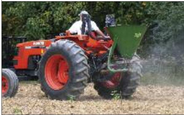
Cyclone seeders cover ground quickly, but are harder to adjust precisely for small seeds.
